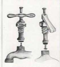
The valve assembly. On most faucets, it is not necessary to remove the top screw and tap handle to fix a drip. Use a smooth-jawed wrench Delightful Accent Pieces
