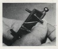
Keep hinges and screws matched in this foolproof way. Slip screws into holes as shown, then fasten closed with a twisted rubber band
