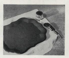
6. Apply one coat of background color. Dry 24 hours, sand, and dust. Repeat as often as necessary to give a smooth surface. Then apply one coat of varnish. Dry 24 hours. Trace on your design, paint with tube oil colors. Dry two weeks. Finish with two coats of spar varnish
