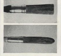
That rounded end is a "chisel" tip. You'll find that it does the neatest and most precise job. However, square ends are satisfactory on big brushes used to paint large outside wall areas
