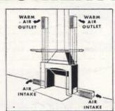
This phantom view of the picture above shows how the Heatilator draws in air at floor level... heats it and circulates warm air to all corners of the room.
