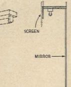
Light up your face at a vanity like this. Fluorescent fixture attached to underside of shelf is masked by plywood strip. All hide behind wooden roll blind. Light doesn't cause glare in mirror because top of mirror is painted color of wall
