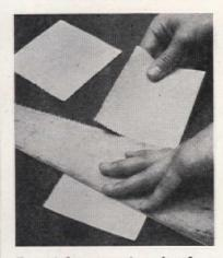
Ever tried to tear a piece of sandpaper? Results-mostly ragged edges. Lay a saw flat on sandpaper, leaving just as much as you need above saw's edge. Rip quickly for clean cut
