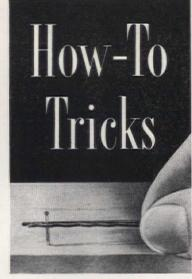
Save your fingers! Hold that small nail or tack with a common bobby pin. Just slip nail through prongs, hold end of bobby pin, and hammer away
