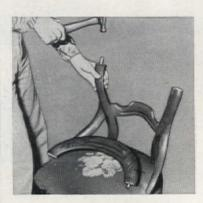
Cut and sand new hickory dowel pin to fit. If pin fit is too snug, chair rail will break because of air and glue compression. To prevent this, flatten one side of the pin slightly with a rasp. Apply glue to dowel pin and hole before inserting pin
