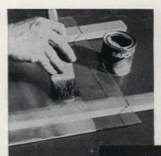
Brush a coat of glass-frosting paint on one side of glass. Keep strokes uniform and brush clear across entire surface of glass
