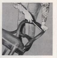
After setting, remove any excess dried glue with a sharp chisel. Fill small open joints with stick shellac. If the joint overhangs slightly, or there is any unevenness, sand flush with 00000 sandpaper. Stain to match original color, and add protective finish to match rest of chair
