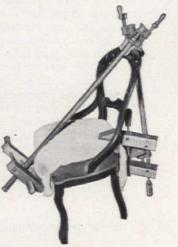
Clamping is difficult because of irregular angle of chairback construction. Force of clamp must be downward at an oblique angle. Note how two pipe clamps are fastened to a board running under chair seat. To squeeze out surplus glue, apply sufficient pressure simultaneously to both clamps. Wipe off glue immediately
