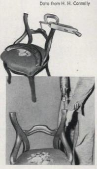
First, make wood repairs which require clamping—for example, a rail which is wholly or partially split. To allow ample time for difficult clamping assembly, use slow-setting resin glue. Protect wood finish with felt or thick cloth between clamp and wood surface. Remove broken dowel pins by drilling with a bit  $\frac{1}{3}$ " smaller in diameter than pin. Remove remaining pieces of dowel with small chisel
