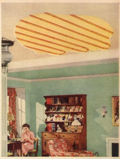
2 Cutaway view shows coils of Bundyweld® Tubing hidden in plaster ceiling. Coils act like sun, send down radiant rays that make you comfortably warm at healthful room temperatures. Heating is draft-free, dirt-free. Redecorating and wall washing are postponed years. Fuel bills are extremely low.
