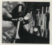
Hold ignition wire to frame and turn engine over by hand. If there is no spark, chances are that the coil is shot
