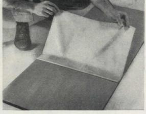
If you are veneering a large panel, it is best to cement it in sections. First lay the veneer carefully over the panel, then fold back half as shown. You apply the cement to the wood, smooth the veneer over the cemented surface, and repeat for the other half
