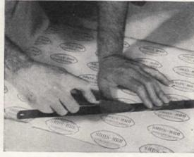
Make paper pattern of each panel. Cut veneer before removing its paper backing. Place veneer face down on hard surface, and cut according to pattern. Use single-edge razor or sharp knife, and guide it with sharp steel edge-top side of hack-saw blade will do
