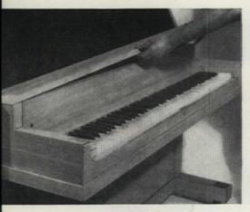
A new piece of wood is used to close the gap which is left after the keyboard cover is installed in its new position
