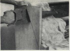
To slant the front, you cut the side panels of the piano this way. First draw a diagonal line from the center of the top of the panel to the point shown here. Then saw along this line. Be sure to protect "works" from sawdust by covering them with a cloth
