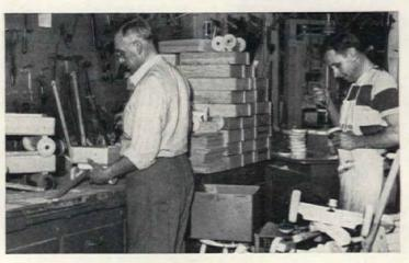
Ed Suhr (left) and Al Wolf, the wagon-making team, go at it in Al's garage workshop. He modified a standard 4" hole cutter to cut the wheel, groove the side, and drill the center hole in one operation
