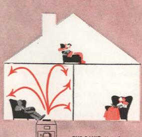
THE FAULT: Heat from pipeless warm-air furnace with single register overheats room where register is located but fails to heat the adjoining rooms or those on the floor above
