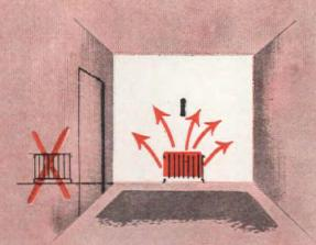
THE FAULT: Improper location of the thermostat near source of heat makes it turn off the furnace before the other rooms in the house have been adequately heated
