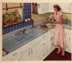
THIS American-Standard sink, with deep compartment and gently sloping drainboards, is made of rigid cast iron with a thick coating of acid-resisting enamel. Comes in white and five beautiful colors. Quality faucet is non-tarnishing, has handy spray.
