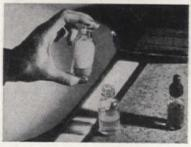
The number of drops of soap required to form suds will indicate the hardness of water in grains per gallon. If more than 4 drops were added, water is considered hard (4 grains per gallon). Water that has been treated by water-softening equipment will produce a good quantity after one drop of liquid soap has been added to it
