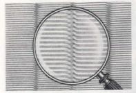
TINY LOUVERS are permanently set at an angle to stop hot sun rays *before* they reach your windows, thus eliminating a major cause of high room temperatures.
