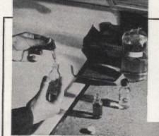
Fill test bottle partially full with water. Add drops of liquid soap, one at a time. After each drop has been added, cap bottle with finger and shake it vigorously. Continue to add drops of soap until a good quantity of lasting suds have been formed
