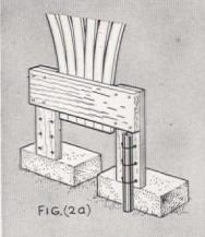
base of a 4-in. crossboard and 3-in.-wide legs 10 in. long; set it on bricks and wire it to pipe
