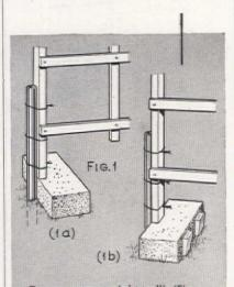
To support a straight trellis (Fig. 1), set each leg on a brick, and wire it tightly to a 2-ft. piece of pipe driven halfway into the ground (1a). To keep bricks in place, drive two wedges or stakes against opposite side of each (1b). For a fan trellis, make a
