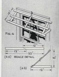
side braces, has the advantages, without the disadvantages, of an awning. Nail three laths 6 in. longer than width of window to three 15-in. crosspieces. Attach wire or cord loop to top of center strip to hook over nail in top center of window frame. For braces, saw 22-in. piece of 1 x 1 wood in half diagonally (4a); nail beveled ends to trellis, and square ends to sides of window frame (4b). To remove in fall, tap braces loose, unhook center supporting loop
