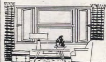
c Showing two Convertible awning sashes, with two casement units. A good combination.
