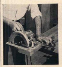
Protractor is a practical guide for making both straight cuts and miters. Angles are set on the protractor by moving the holding arm to desired degree mark. It can be used on either side of saw
