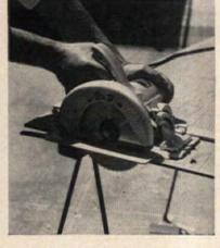
Blade depth can be corrected by adjusting the thumbscrews at the front and rear of the saw. If saw binds or stops, hold power switch on, and back saw down the cut until motor starts to run again
