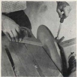
DISK SANDER allows work to be held stationary on saw table. Secret is that the quill can be used to move the disk into the work. For exact duplication, the miter gauge can be locked in its slot by tightening a built-in expansion bolt. Using table's tilt features and miter would allow you to sand compound miter joints
