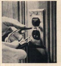
Always connect grounding wire before inserting power plug. A special screw that comes with saw converts most household outlets that are grounded, to convenient grounding outlet for the saw
