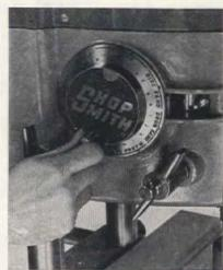
Speed dial, built in headstock, gives 675 to 6200 rpm speed range. It's important to have because different operations must use different operating speeds
