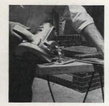
Compound miters are cut by making use of the bevel angle adjustment on the saw and by using the protractor as a guide on the work. Protractor is also useful for laying out general carpentry to be done around the house
