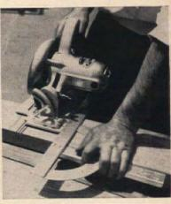
Cut dadoes by making outside cuts first and cleaning out remaining wood with a chisel or by making a series of close parallel cuts. Use of protractor keeps cuts in alignment as you make them
