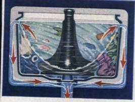
An activated "float-away" rinse flushes out 1003ened soil. And in the spin, dirty rinse water is lifted up and over edge of washbasket, safely away from your wash, not strained through your clothes as in many washers with holes in the bottom of the tub.
