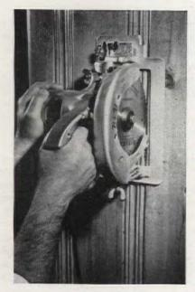
Pocket cuts on existing siding or flooring should be made with a special nail-cutting blade. Make the cut by placing the front of the shoe on the work, rest teeth lightly on work, start motor, and with blade running, lower saw into work until shoe is flat. Then move saw forward to make the cut
