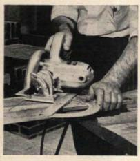
Miters are easy to cut if you take advantage of the scale on protractor. You can use the protractor to cut angles of any degree, as it is adjustable for almost a full 180° swing
