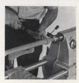
LATHE was used for turning clock columns and can handle work to 34-in. long with a 16½-in. swing. Cup center in tail stock can be offset up to ½ in. for taper turning. The tool rest sets in the saw table carriage and adjusts for height with a lever and slides on the main ways to any location between the lathe centers
