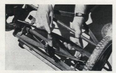
Once your mower is really clean, coat the cutting edges (both moving and stationary blades) with heavy oil or cup grease to prevent rusting, which means heavy pushing, poor cutting, and unpleasant noise next year. An old paintbrush and oil drained from your automobile crank case come in handy for this job MORE ON PAGE 140
