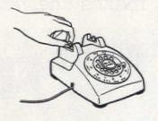
**cut-off switch:** pulling up the special knob temporarily cuts off extensions on same line, so no one elsewhere in home or office overhears your conversation.
