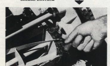
Freedom from picked-up grass is especially important with chain-driven power mowers. Try to keep moving parts clear all the time, after and during use. A good tool for this is a sharpened hook of #9 wire with a ring in the other end so it can hang handily from your belt or the handle of the mower
