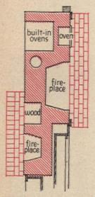
Two fireplaces are backed up (staggered on plan) in single masonry wall. Build one, or both, to remodel your present living room, or to add a new room
