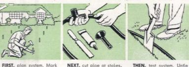
NEXT, cut pipe at stakes, roughen ends. Cement fittings to pipe. Tie heads to stakes.
