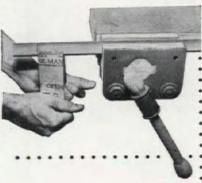
Round and odd-shaped pieces are often easier to sand with narrow strips of sandpaper used as shown. You can also buy sandpaper and abrasive cloth in rolls of various widths. It's handy for getting at difficult spots
