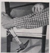
Tight clamping makes stronger joints. To clamp chair rungs, tie cord around legs, loop it, insert hammer handle, and twist to draw rope tight. Do same to repair irregular-shaped objects.
