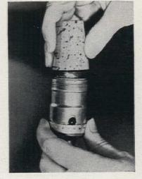
You can remove a broken bulb from a socket quickly and easily with a large cork. First, turn current OFF. Then press the end of the cork onto the base of the broken bulb and turn the cork counter-clockwise. That does it!
