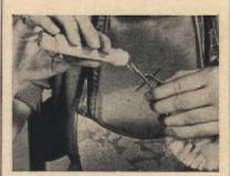
To tighten loose handle on a household brush, remove handle and spread twisted wire with a large nail. When replaced, handle fits snugly over tang.
