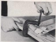
When using clamps, always protect the surface of the joint with a heavy pad of newspaper or two pieces of scrap lumber on each side of joint to prevent leaving clamp marks on work.
