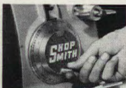
SPEED-DIAL —Instant selection of correct tool-speeds. Exclusive Power-Shift from 700 rpm to 5200 rpm!
