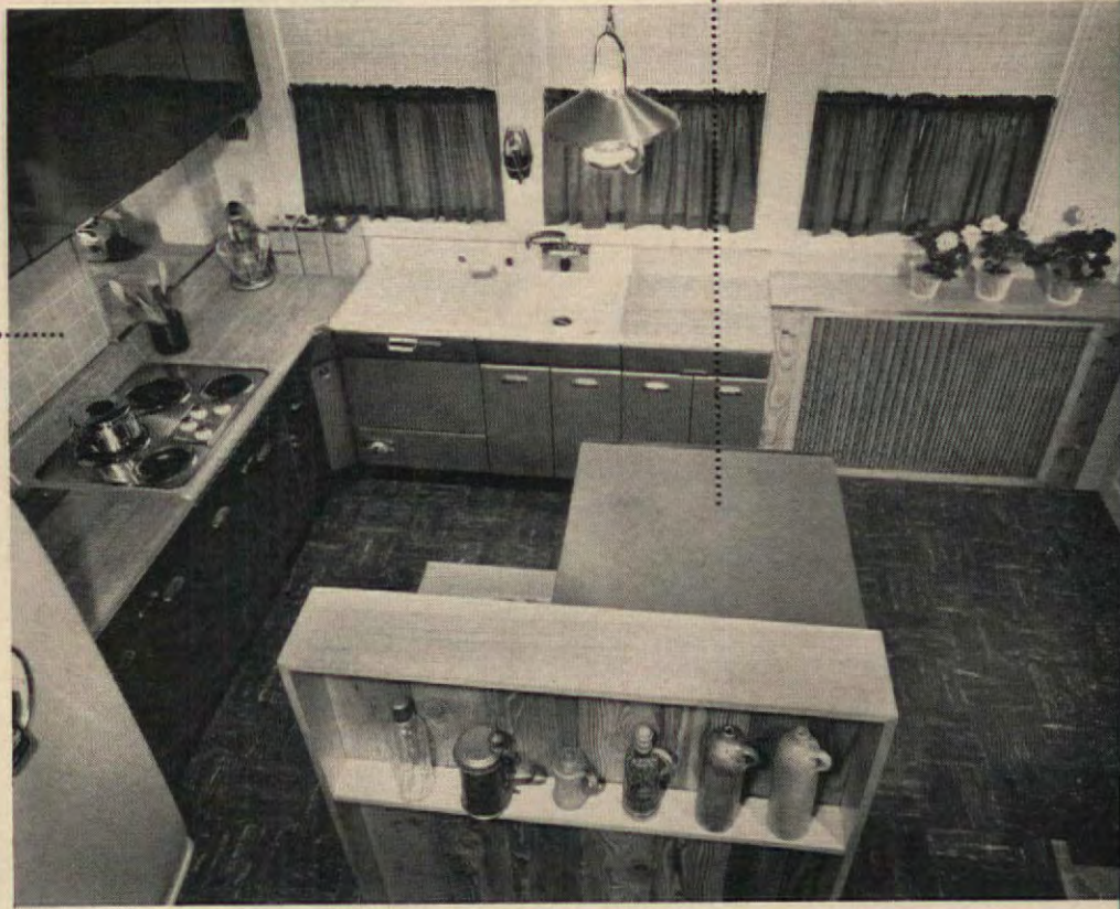
Here's a ceiling-to-floor view of the kitchen. Notice how the stack-on oven and its counter form island to free work area from flow of traffic (above). There's a roll-out waste basket under the counter at end of island (top). Made of perforated hardboard, it's painted to match cabinets.
