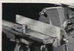
POWER-MOUNT —for attaching jointer, band saw, jigsaw, belt sander and sprayer. Another SHOPSMITH exclusive!
