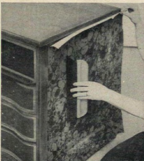
7. Brush paper with a smoothing brush to remove any air bubbles. If bubbles do appear, loosen paper at corner, brush from center to corner.
