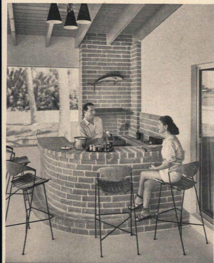
At your service . . . this built-in barbecue bar. The grill of pink slump brick was designed by Mr. Taub, the niche built in to accommodate a standard size grill. Cabinets underneath bar store necessities—among them an electrically-motored attachment for the rotisserie.
