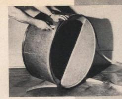
Now bend 16"-wide untempered hardboard strip around top, bottom. Tie in place. Use 1" nails 2" apart to fasten bottom flush, top  $\frac{1}{2}$ " below edge.
