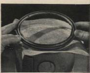
Strain paint quickly by this method. Use scroll saw or tin snips to cut center from lid of old can. Use this "donut" to hold cheesecloth in place.
