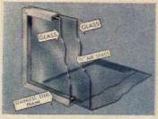
METAL EDGE. These units are designed for larger window areas and where maximum insulation is needed. They are constructed of two panes of ¼" clear-vision Plate Glass, with a ½" sealed air space between them. The exclusive stainless steel frame protects the glass against chipping, creating very strong units.
