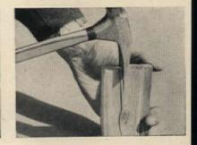
Like a hatchet it splits wood when rough-shaping demands it. If ends of claws are kept sharp, you can even point the ends of stakes, too.
