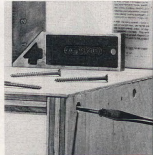
Invisible corner easiest to make is deep rabbet which leaves only one-eighth inch of top showing. Fasten with glue and screws driven at slight angle.
