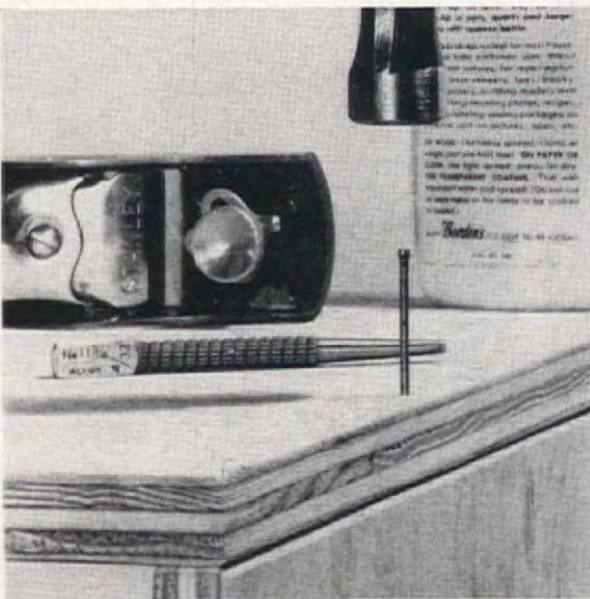
Butt joint is simplest and one of the strongest if it is well fitted and glued as well as nailed or screwed. Plane V-groove where two members meet so joint will become part of design.
