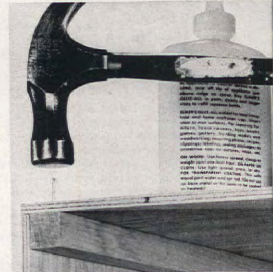
Cleated corner is only answer when you use thinner plywood which isn't bulky enough to fasten to itself. Joint is very strong when 1x1 cleat is used.
