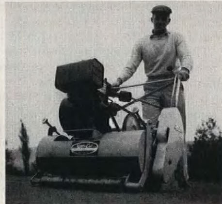
Verti-cutting with this machine is a new phase in bentgrass maintenance. It cuts the runners to produce a thicker turf and is done two or three times a year.
