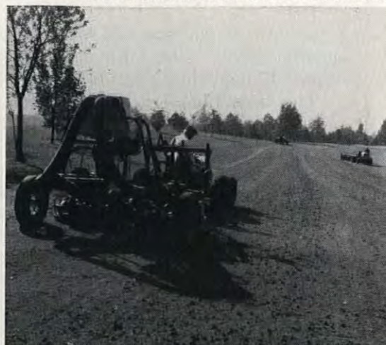
This giant verti-cutter is used after aerating to break up the soil cores left by aerator, and to cut the runners of bentgrass turf.
