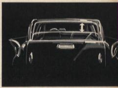
No clumsy two-piece tailgate. Rear window rolls down, can be controlled by driver.
