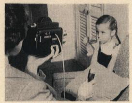
SOUND IS ADDED to home movies with this 8 mm. camera that picks up and records sound and action simultaneously on the same film. Developed by Fairchild Camera & Instrument Corp., Yonkers, N.Y., camera and microphone are \$239.50, its projector-recorder, \$249.50.
