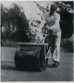
Rolling is done in early spring and a few times later. The empty power roller is about equal to a half-filled home model.
