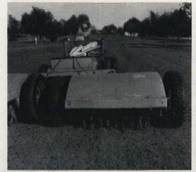
Fairway aerator punches holes in the turf to increase aeration, water penetration, and reduce "thatch." It's used twice a year.
