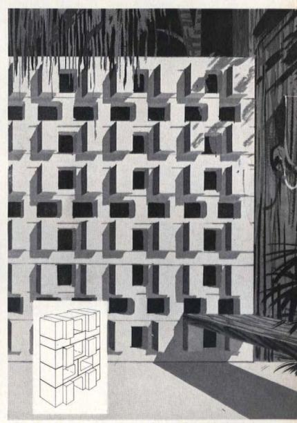
Partition blocks and lintels form this complex, projecting design. A job for an expert. Following the sketch, the basic units are: partition blocks in 4x8x8" and 4x8x16" sizes; lintel blocks, 8x8x8". Shopping Information, page 81
