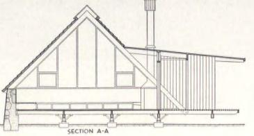
Section of living room shows how "A-frame" virtually eliminates the need for outside walls. This type of construction is becoming very popular because of its economy and also because in a cold climate it sheds snow easily, eliminating the need for a heavily reinforced roof frame.
