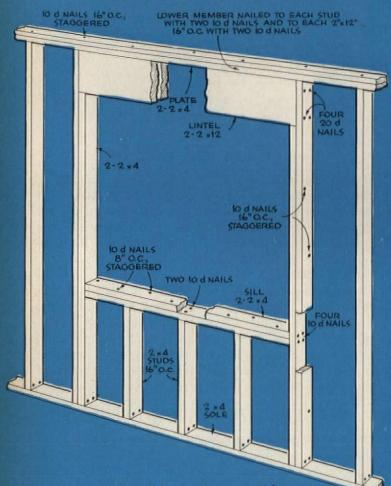
A window over 3' wide which comes to 10 or 12" from top of wall requires a wide lintel (header). This can be made from two pieces of 2x12 or 2x10 to simplify framing.
