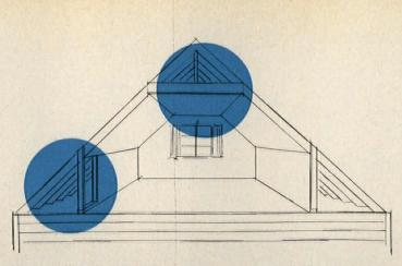
Knee-wall and ceiling framework are required if an attic is to be finished into livable quarters. Simplest way to bring materials into the attic is to hoist them up through the attic window.
