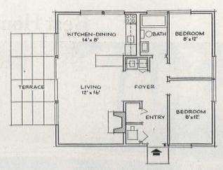
**One-floor plan** for the cabin on top of page 48 is both roomy and efficient. This is a year-round vacation house. Closet just inside front door houses furnace. House is variation on a standard plan designed by Carl Koch, A.I.A.
