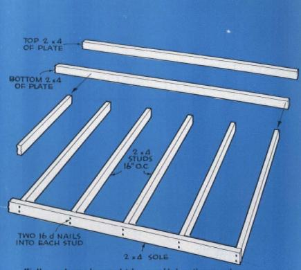
Wall panels can be completely assembled on the ground or floor, with the exception of the top member of the plate, and then tilted into place and secured when plumb.
