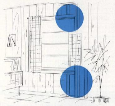
**Panel construction** requires doubling up of lintels and side pieces of all openings. Studding should also be doubled where panels join. Plan openings to fall in center of panel.
