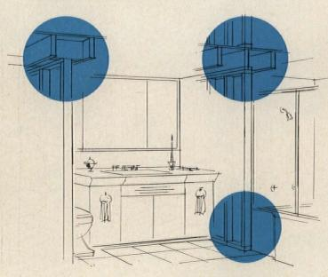
Interior partitions must be solidly connected at both top and bottom to prevent any movement of the wall. Use masonry anchors to connect sole to concrete floors. If the partition runs at right angles to the joists, you will have no particular problem in tying the top of it to the ceiling. Even if the ceiling has a finish of wallboard or plaster, you can spike the top plate directly into the joists without any great damage.
