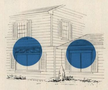
Rough openings for windows must have adequate support along the top to prevent the top plate of the wall from sagging. This can jam a movable sash and crack the glass.
