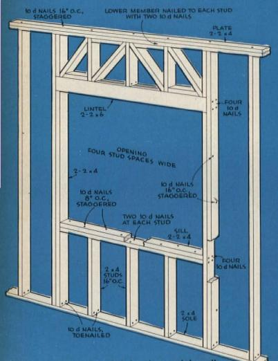
For a window more than 12" below the top of the wall, use the above method of framing with the lintel made (continued)
