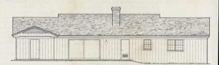
An attractive rear elevation, as carefully designed as the front, doesn't have that "back-yard" look. Sliding glass doors lead from the patio into the family room. Door at left leads to storage, breakfast-kitchen area.
