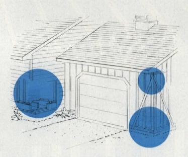
Sills and corner posts of buildings must be level and plumb. If an existing sill is not level to begin with, put a thin layer of mortar on top or use wood shims.
