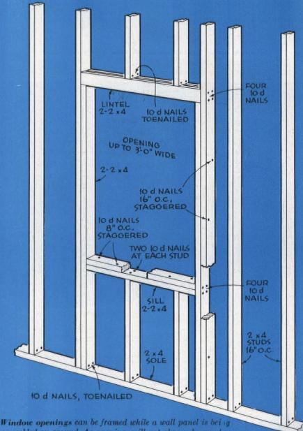
assembled on ground. As openings will not always be equal to standard stud spacing, use intermediate studs where necessary
