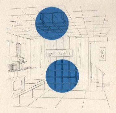
**Framework is required** for basement walls and ceilings. After all framework is in place, apply the ceiling material and then the wall covering.
