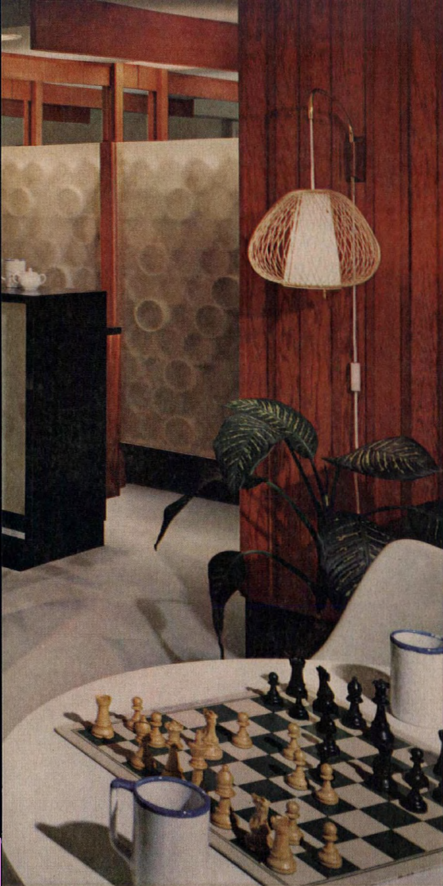
Dramatic built-in bar of walnut veneer is faced with the same plastic fabric which covers the bar stools. The decorative circle design behind the bar was created by stacking and gluing fiberboard tubes in 4", 5", and 6" lengths, then placing the tubes behind five plastic panels.
