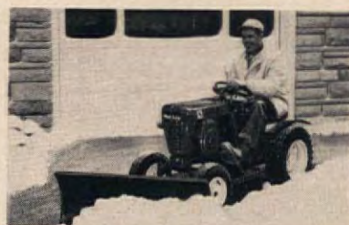
Snow-Blade. An attachment also useful for earth grading. Other attaching tools include snow-thruster, reel mowers, rake, lawnsweeper, spreader, steel dump trailer, and utility wagon.
