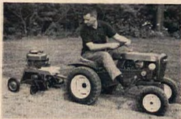
Self-Powered Tiller. A Wheel Horse attaching tool for the serious gardener. Has own 5½ hp. engine. Designed to dig deep through hard packed earth. Other garden tools include plow, cultivator, disc.
