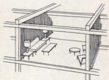
Heart of the "Space Frame" concept is basic 16-ft. x 16-ft. unit of construction (called a "module") shown in diagram. Any number of these can be linked together and enclosed in any pattern desired to create living areas.
