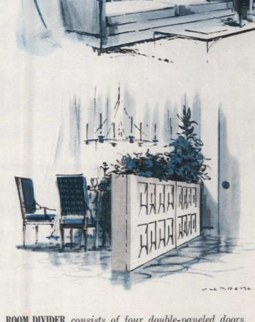
**ROOM DIVIDER** consists of four double-paneled doors. Each side has two doors laid lengthwise. Keep sides far enough apart so lips of planter boxes will rest on edges of doors. Fasten doors to floor with angle cleats two to a door. Cover the open end with clear pine board.
