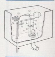
The working parts of a toilet tank: 1. flush valve hole, 2. flush valve hole seat, 3. flush ball, 4. connecting rod, 5. connecting linkage, 6. handle linkage, 7. handle, 8. guide arm, 9. overflow tube, 10. float rod, 11. float, 12. valve screw, 13. valve plunger.
