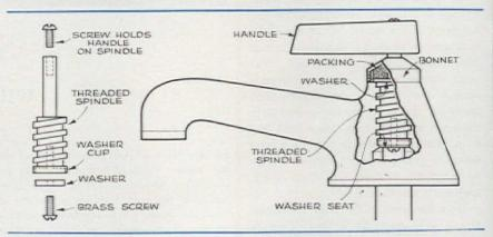
or in a kitchen faucet around the base of the swing spout, the packing or the O ring may need replacement.
