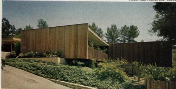
The site was graded only enough to receive the house which cantilevers over hillside. Extended foundation wall became a planter. Exterior is weather-resistant redwood. Unpainted fence blends into landscaping unobtrusively.
