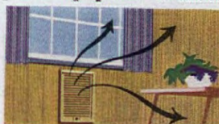
Wall panel, with heating units behind grille, provides radiant heat with natural or fan-forced convection.
