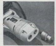
spindle, it has two, each with a choice of two rotation speeds. Thus, by placing the chuck on either spindle, and varying the speed of that spindle, you get a total of four speeds. Chuck capac-
