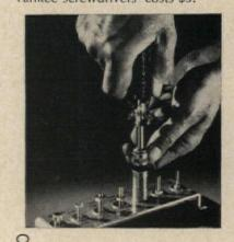
Mounting cabinet hinges becomes an easy job with the Vix-Bit, a selfcentering tool which fits the chuck of an electric drill. Pressing the tapered front into a hole in the hinge centers the built-in drill. Increasing
