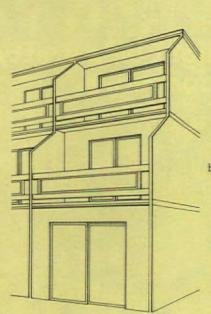
Factory-built housing needn't be homely. The units shown left, built in Oakland, California, by Building Modules, Inc., house people earning \$8000 or less per year. Each section, 12 by 12 by 8 feet inside, is cast in concrete, then lowered into place with bathrooms, kitchens, and most partitions already in. Once stacked, premanufactured parts are added to complete each unit. Compared to conventional methods, estimated savings are one to three dollars a square foot.
