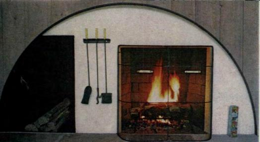
big-wall fireplace (left), he avoided expensive materials (such as stone) and simply framed an arched opening in the wood wall with a steel band and stuccoed the concrete-block chimney. He used a normal-size fireplace opening but combined the log storage space and fire implements into a single composition to fit the scale of the room. The hearth is bluestone.
