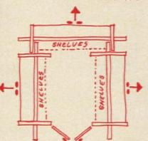
Slotted construction provides stability without framing; 1-by-4's join panels and support shelves.
