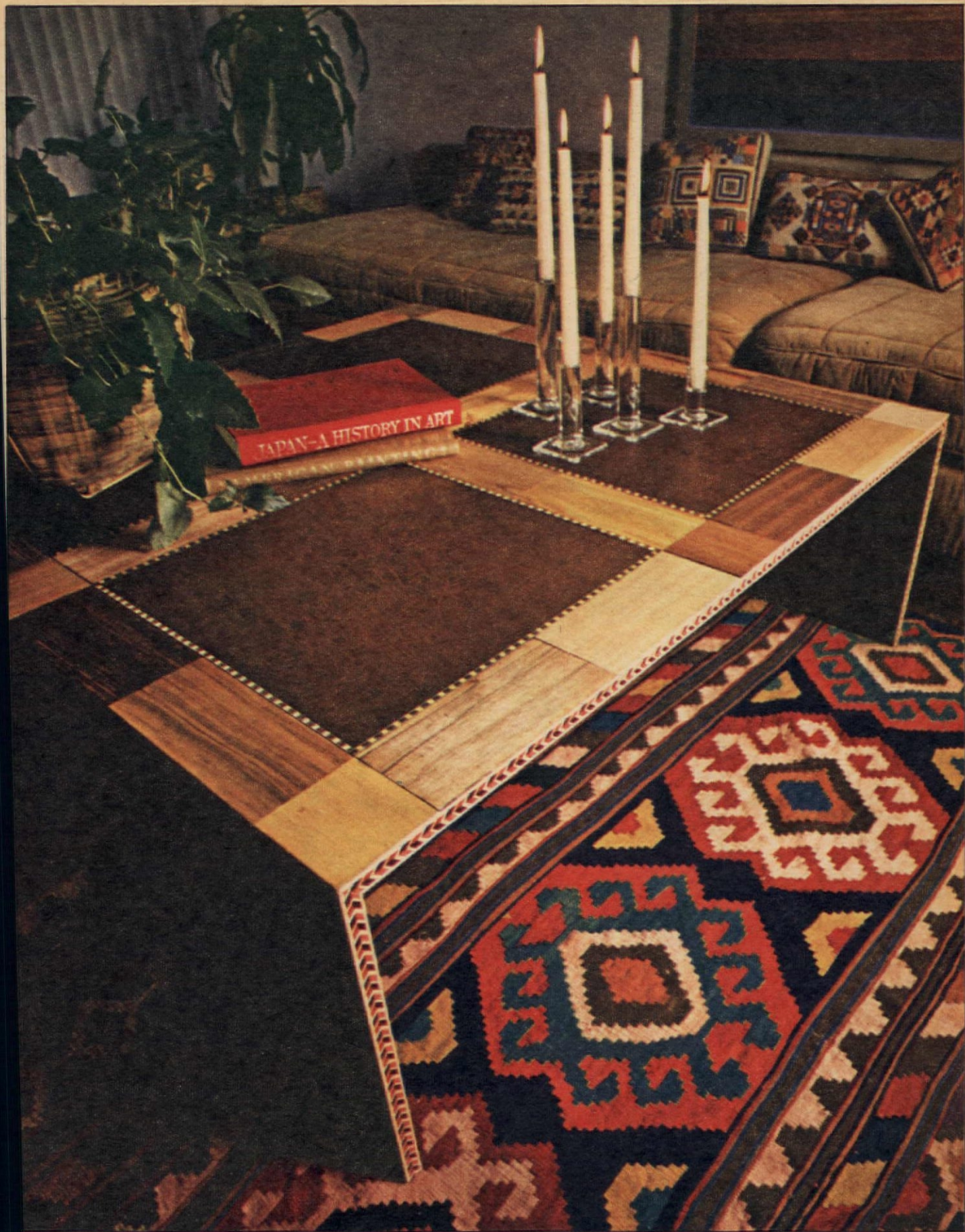
Three-quarter-inch plywood is the basis of this marquetry table. After constructing table, we marked out design. Wood veneers and self-stick paper were applied, accented by inlay strips also used as table edging. Instructions are in "Table Talk," page 28. Total cost: about $40.
