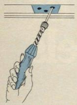
There's a new version of that old favorite, the ratchet screw driver. It has a spring, self-return drive that can be reversed when you need to pull screws out.
