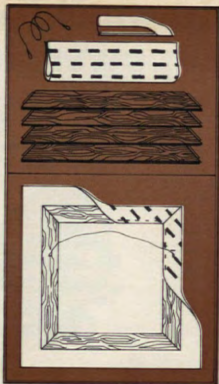
Top: materials—staple gun, picture wire, stretcher bars, and sheet. Bottom: miter corners; staple, attach wire.
