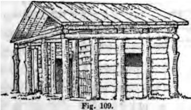
The trunks of trees, set perpendicularly to support the roof, may be taken for columns; the tree laid upon the tops of the perpendicular ones, the architrave; the ends of the cross-beams
