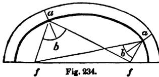
330.—To find the direction of the joints for an elliptical arch. A joint being wanted at  $a$ , (Fig. 234,) draw lines from that point to the foci,  $f$  and  $f$ ; bisect the angle,  $f a f$ , with the line,  $a b$ ; then  $a b$  will be the direction of the joint.
