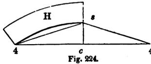
equal to  $c4$  in the previous figure, and  $cs$  equal to  $cs$  also in the previous figure ; then describe the inner edge of the board,  $H$ , according to *Art. 87* : the outer edge can be obtained by gauging from the inner edge. In like manner proceed to obtain the next board—taking  $p5$  for half the chord and  $pn$  for the height of the segment. Should the segment be too large to be described easily, reduce it by finding intermediate points in the curve, as at *Art. 86*.
