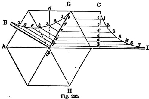
312.—*To find the shape of the angle-rib for a polygonal dome.* Let  $A G H$ , (*Fig. 225*), be the plan of a given dome, and
