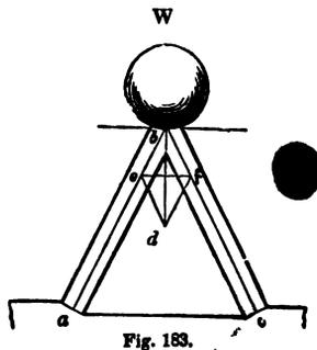
for the weight would be in that line. But, as it rarely occurs in systems of framing that weights can be supported by any single resistance, they requiring generally two or more supports, (as in the case of a roof supported by its rafters,) it becomes important, therefore, to know the exact amount of pressure any certain weight is capable of exerting upon oblique supports. This can be ascertained by the following process.
