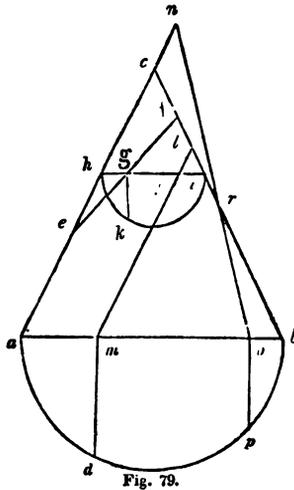
cone be cut by a plane in the direction,  $ef$ , the section will be an *ellipsis* ; if in the direction,  $ml$ , the section will be a *parabola* ; and if in the direction,  $ro$ , an *hyperbola*. (See *Art.* 56 to 60.) If the cutting planes be at right angles with the plane,  $abc$ , then—
