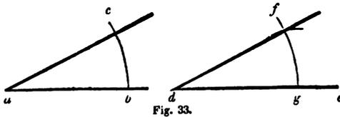
76.—*To make an angle, (as  $e d f$ , *Fig.* 33,) equal to a given angle, (as  $b a c$ .)* From the angular point,  $a$ , with any radius, describe the arc,  $b c$ ; and with the same radius, on the line,  $d e$ ,
