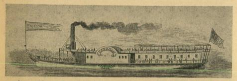
Steamer "Paragon" was the 47th boat on Western waters. Built in 1819 she retained some of the characteristics of the first boats—bowsprit, transom and awning-shaded passenger deck. The berths, however, were above deck, as were the boiler and engine.
