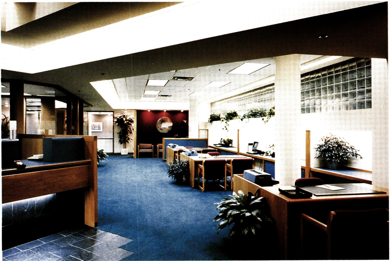
At Honolulu Federal Savings and Loan Association in Kahala, fluorescent coves for vertical and task lighting were used with incandescent accent lighting. Photo by Augie Salbosa
