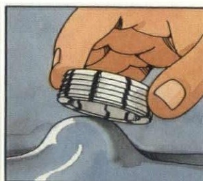
2 Roll and snap on white retainer clip.
