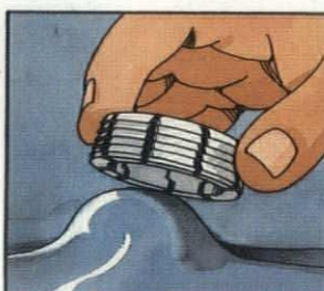
2 Roll and snap on white retainer clip.
