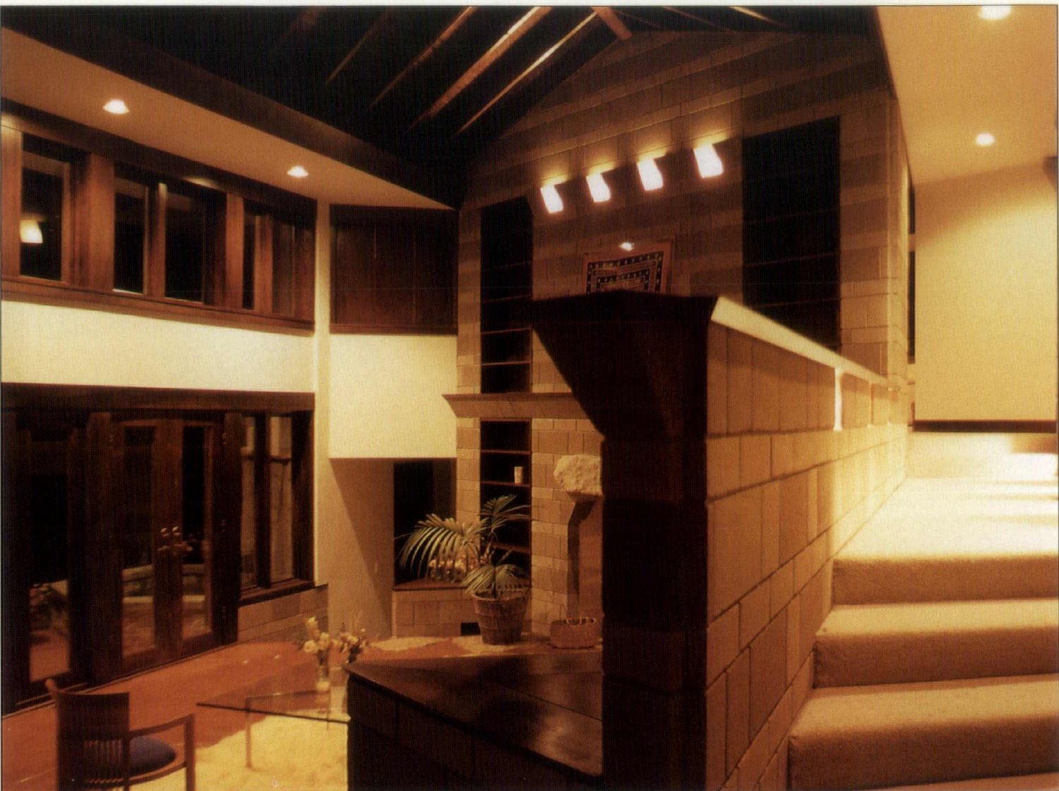
Above: The splendid double height living room and gallery sits on 90 tons of sand for thermal storage and is highlighted by a 2-story lookout tower that also performs as a cooling chimney. The use of exposed framing and alternating bands of concrete block creates an inviting place to admire the entire home.
