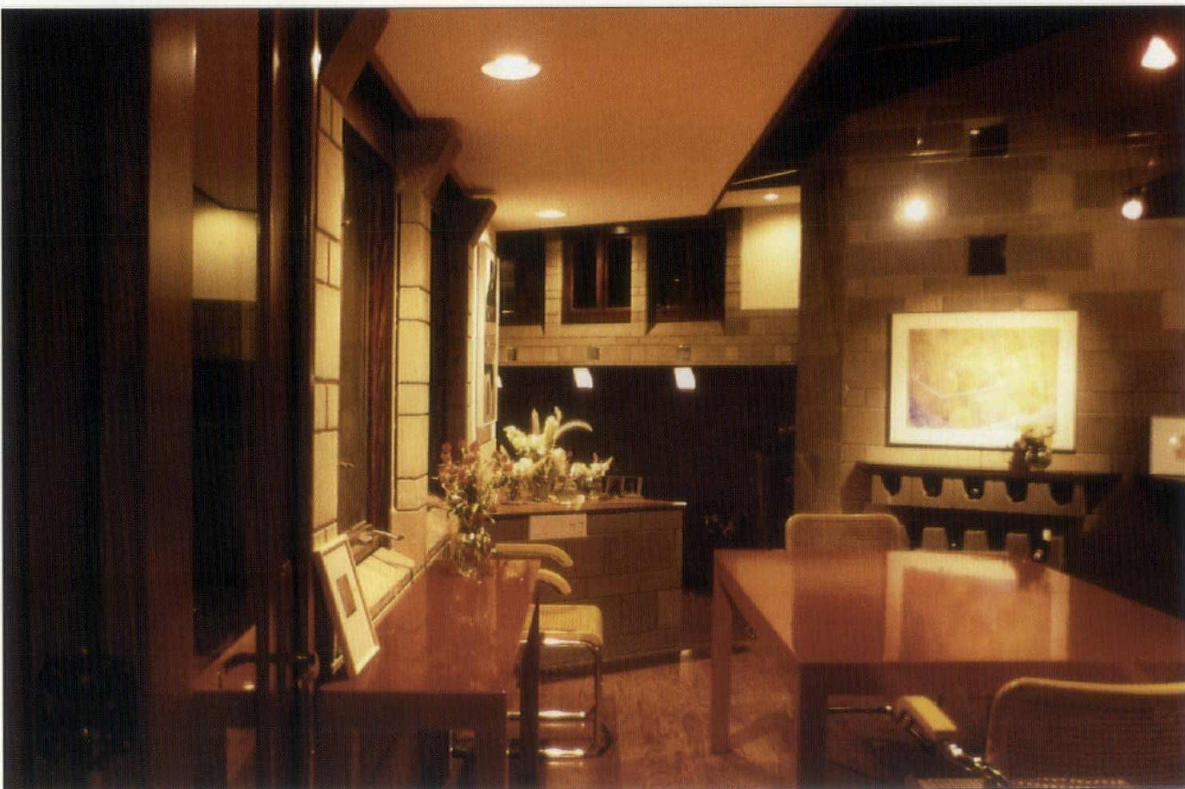
Above: The splendid double height living room and gallery sits on 90 tons of sand for thermal storage and is highlighted by a 2-story lookout tower that also performs as a cooling chimney. The use of exposed framing and alternating bands of concrete block creates an inviting place to admire the entire home.
