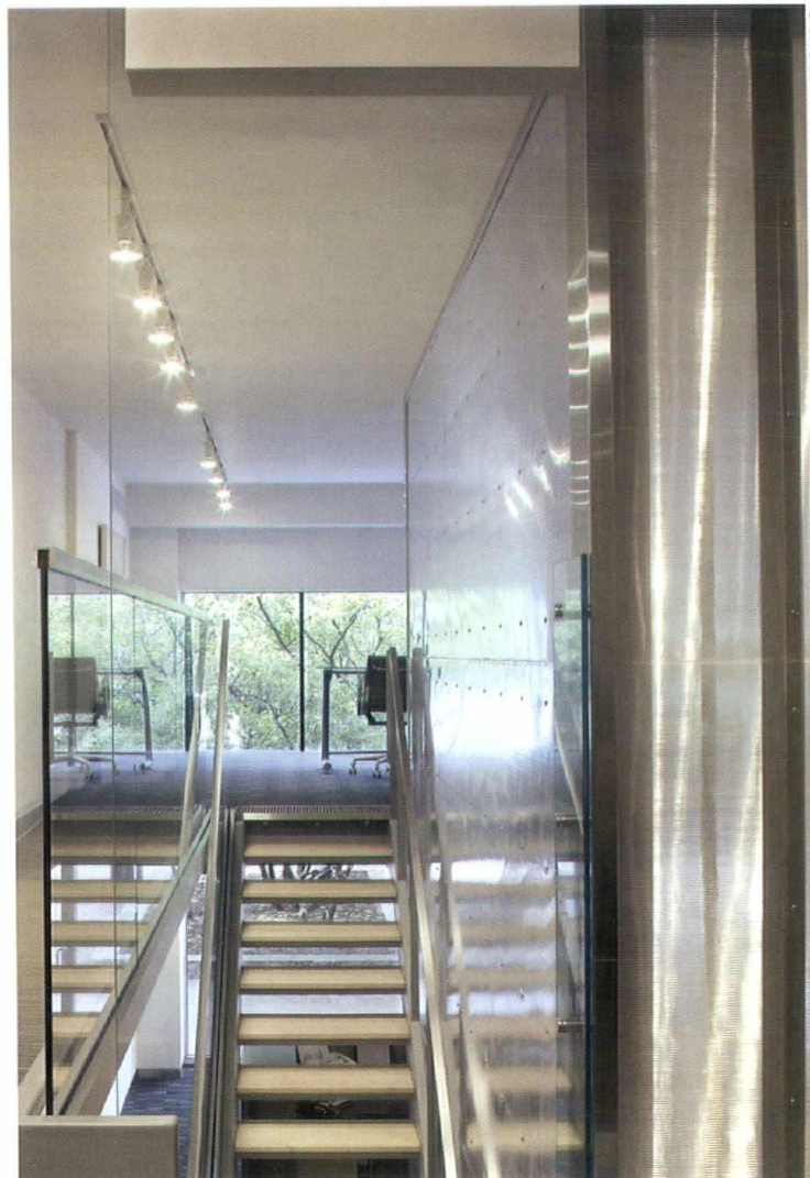
Above: Inside the central conference room, polycarbonate panels provide privacy but also allow the transfer of natural light.
