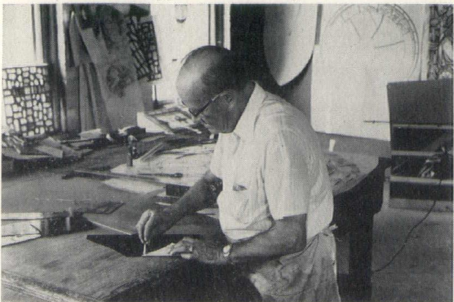
3. Patterns made from the full-size drawing are used to cut each piece of glass to shape. The patterns also indicate the color of glass needed.
