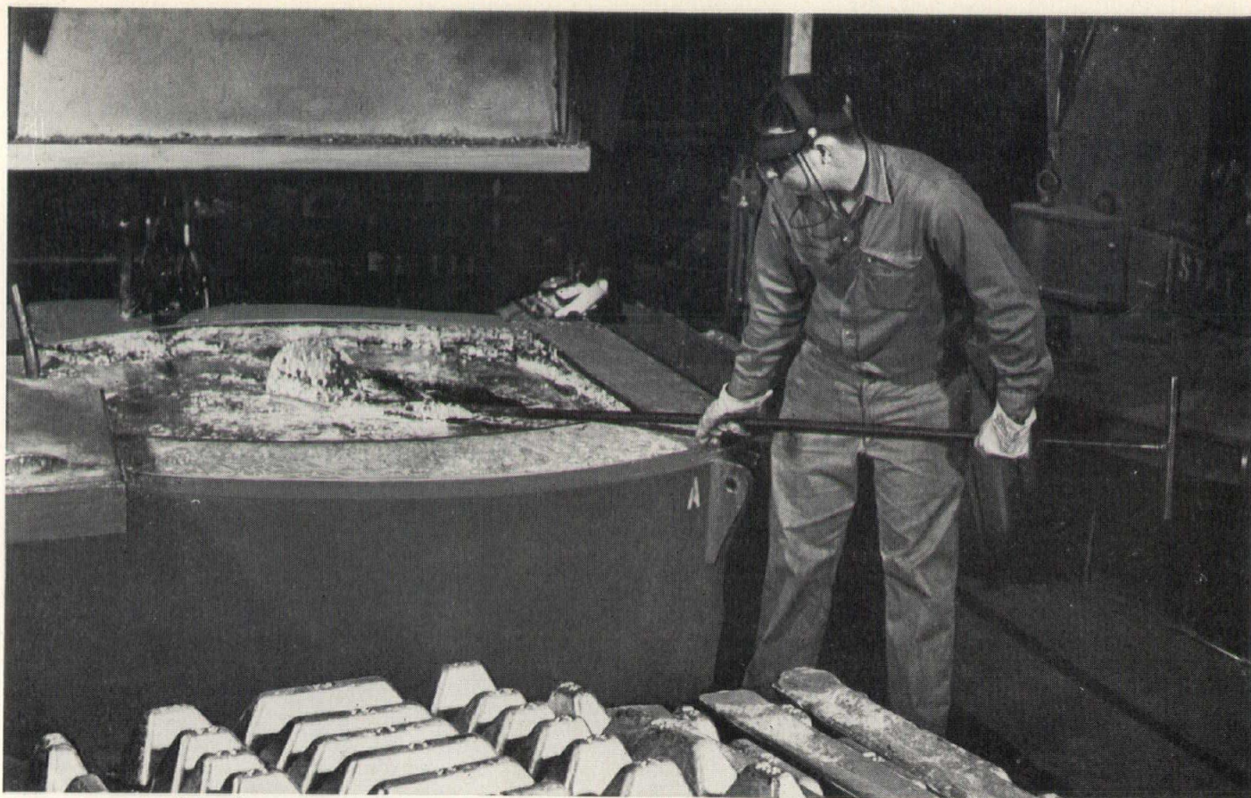
A low-frequency induction electric melting furnace at the Butler, Indiana, plant of Bohn Aluminum & Brass Corporation
