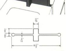
The new WF Blok-Joint is specifically designed to simplify and speed the caulking of the joint in 8" block walls. The wide flange fills the joint to within  $\frac{1}{2}"$  of each face of an 8" block wall, thus forming a convenient dam to permit complete filling for proper sealing. Inadequately thin or wastefully thick caulking is avoided.
