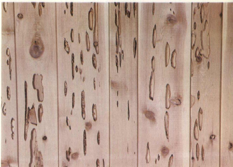
SMOOTH — Surface is smooth with particles left in pecks.
