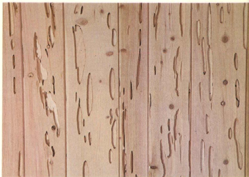
SAND-BLASTED — Textured surface with particles removed from peck
