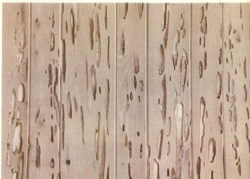
RE-SAWN — Horizontal saw marks visible with particles left in peck
