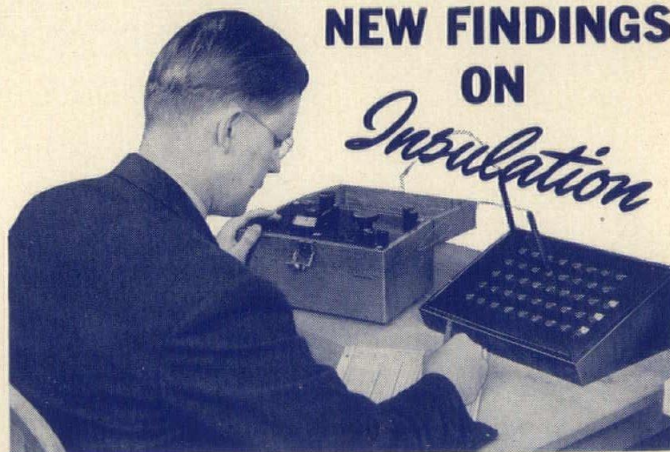
Taking temperature readings at 43 thermocouples with potentiometer.
