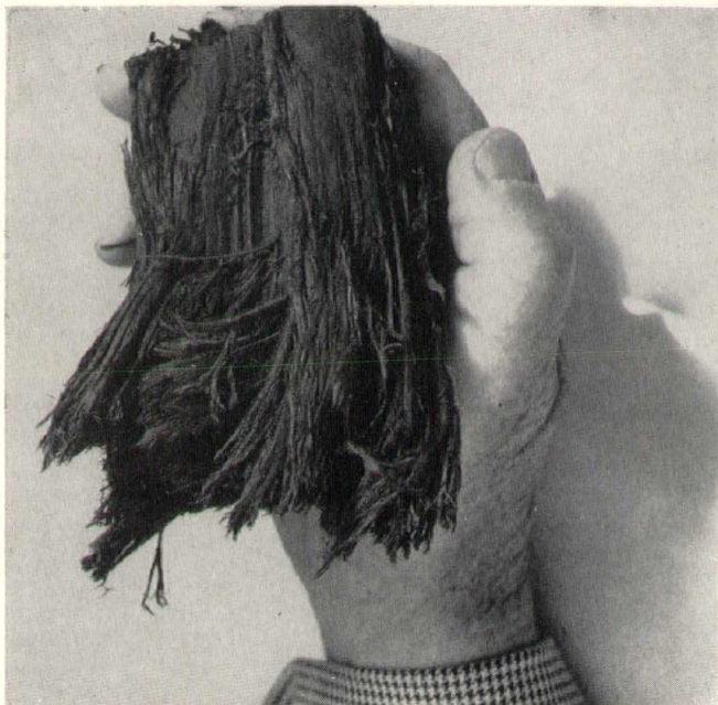
Above: Redwood fragment from 260-foot depth is frayed by well-drilling bit.
