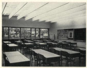
Manufactured light (above) provides adequate levels of light in this room and four-foot windows allow good visual association with outdoors. . . . Four-foot overhang (right) provides sun shielding for sun altitudes down to 45°. Shades draw up for further darkening.
